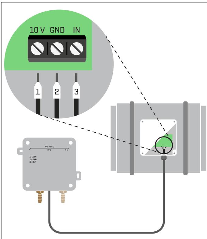
Fig. 2: Electrical connection of the device
