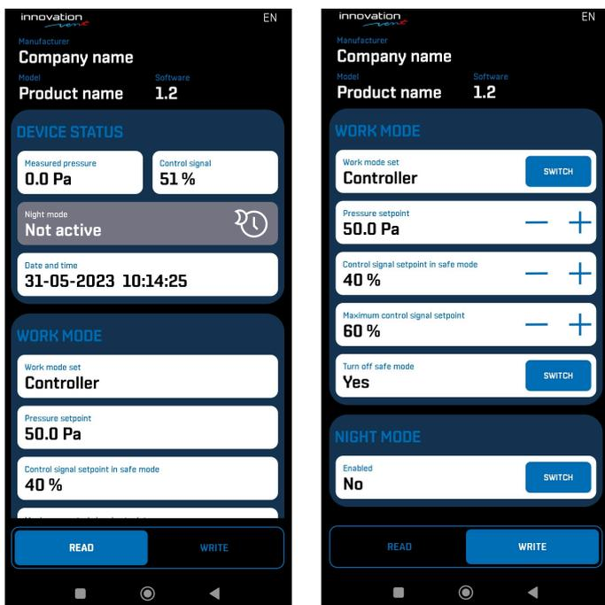
Fig. 6: 'Read' and 'Write' tabs
